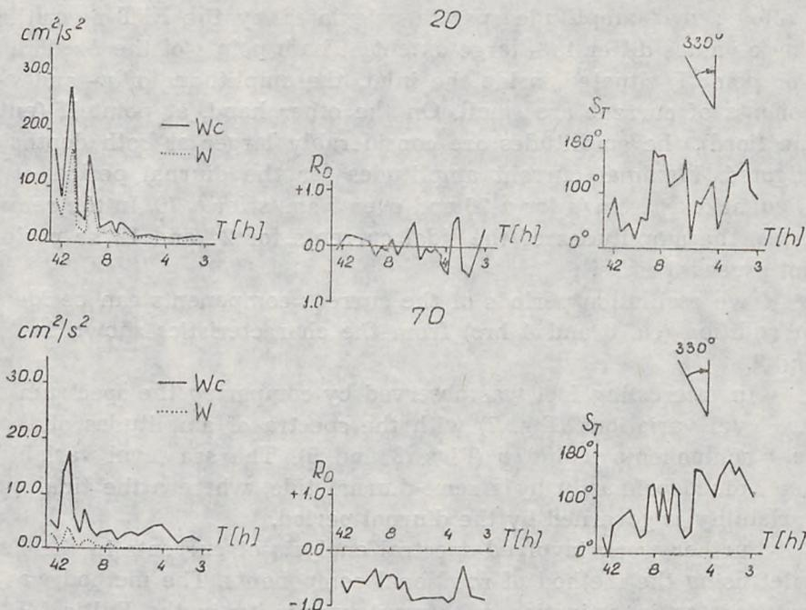
Fig. 10. Rotational spectrum  $W$ , rotation coefficient  $R_0$  and orientation of the major axis of ellipse  $S_T$  of currents at point I
