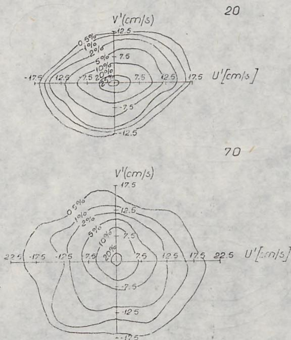
Fig. 5. Two-dimensional distributions of current pulsations at point I (depths 20 and 70 m)
