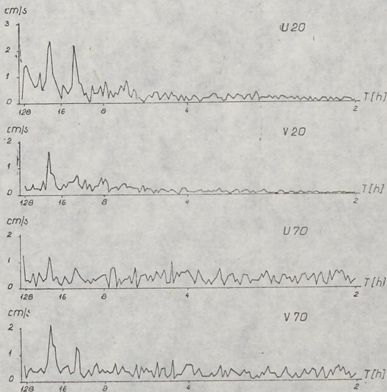
Fig. 8. Amplitudes of periodic oscillations of the current components at point I (depths 20 and 70 m)
