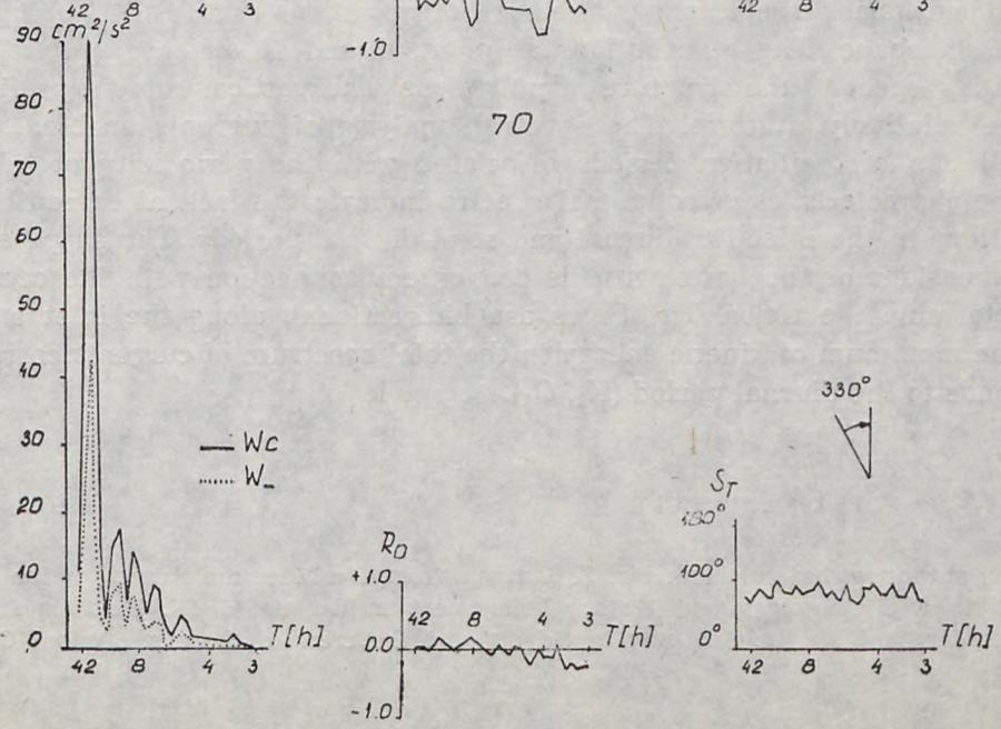
rotation coefficient was  $R_o = -0.5$ . This phenomenon is probably due to characteristic bottom relief at point I. The relief is determined by the 100 m isobath from the east (perpendicular to the inlet axis) and Dufayel Island from the west. The currents at this point contribute relatively little kinetic energy to the spectrum.
