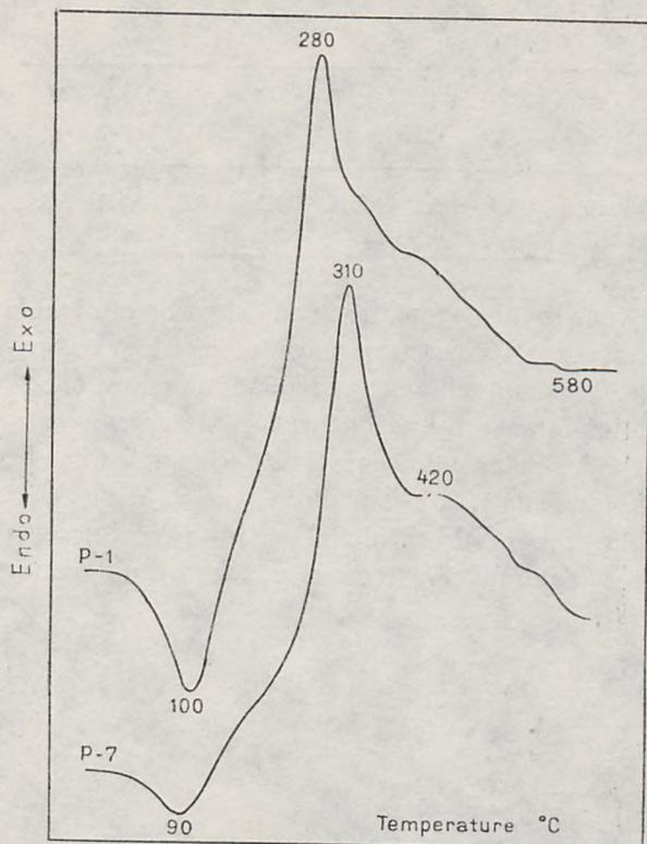
Fig. 4. DTA curves of samples P-1 and P-7
