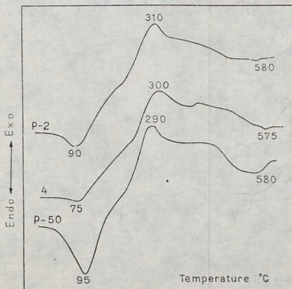
Fig. 2. DTA curves of samples 4, P-2 and P-50
