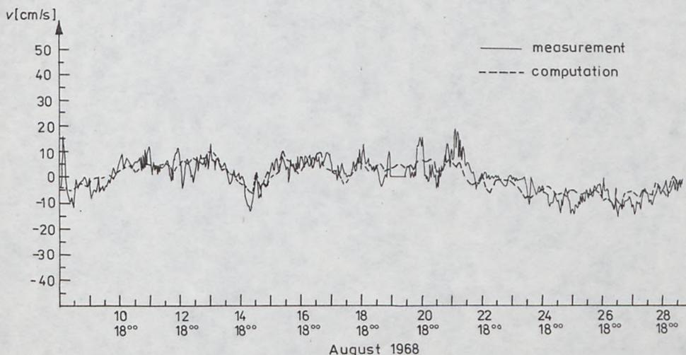
Fig. 4. Normal-to-shore component of the current according to measurements and computations for Hel measuring point
