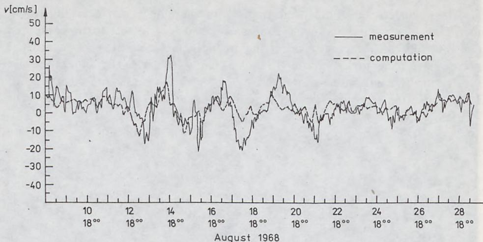
Fig. 5. Along-shore component of the current according to measurements and computations for Hel measuring point
