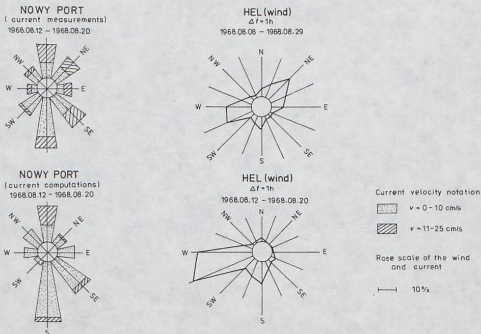
Fig. 6. Current roses of the measuring point at Nowy Port, according to the measurements and computations. Wind roses at Hel for the periods of measurements
