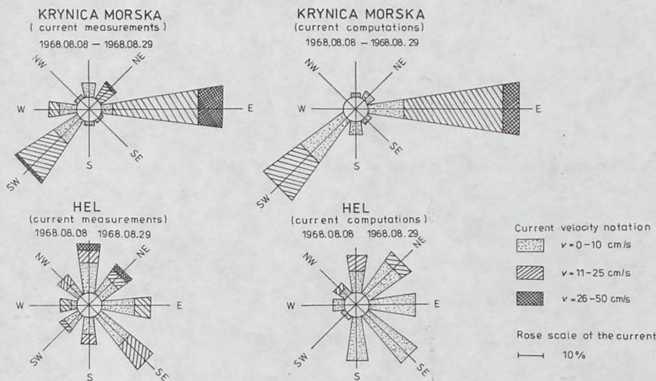
Fig. 3. Current roses of the measuring points at Krynica Morska and Hel (according to measurements and computations)
