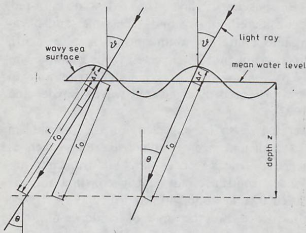
Fig. 2. Geometry of the source mechanism for irradiance fluctuations associated with fluctuations in path length
