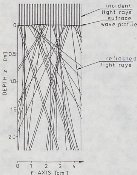
Fig. 5. A complex pattern of light rays under realistic profile of wind-generated water waves in the gravity-capillary transition region
