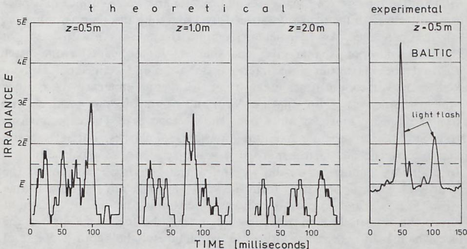
Fig. 6. Calculated light intensity curves for selected depths having intensity peaks due to the focusing produced by a wave profile shown in Figure 5. For comparison, a typical sample of *in situ* record of downward irradiance fluctuations is also shown
