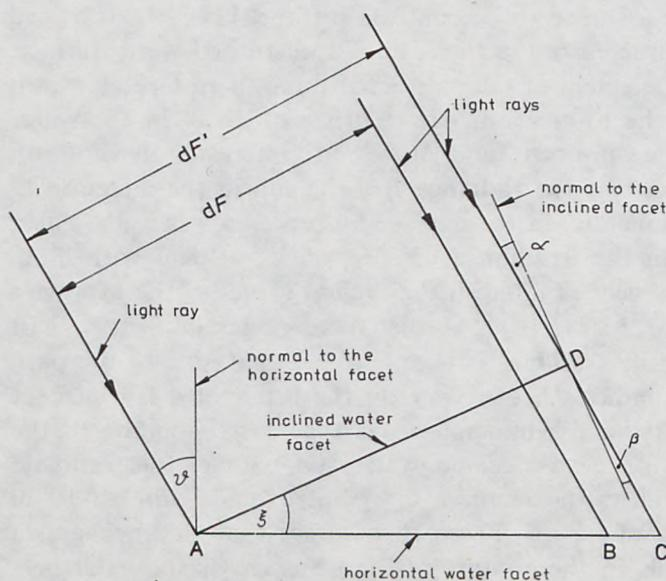
Fig. 3. Geometry of the source mechanism for irradiance fluctuations associated with fluctuations in slope of a water facet
