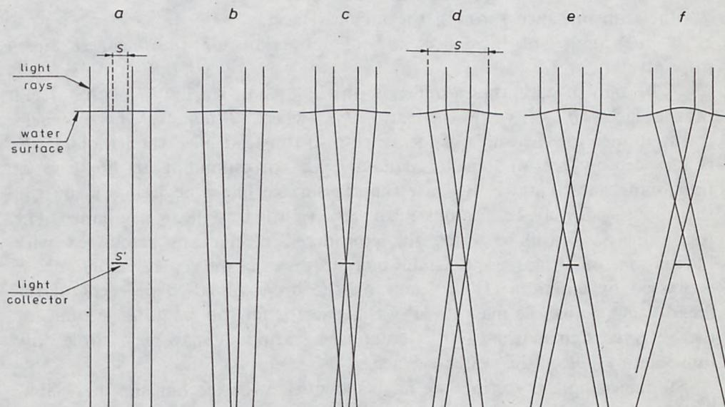
**Fig. 4.** Schematic details of sunlight focusing by wave crest for a light collector of fixed size placed at a fixed depth.
