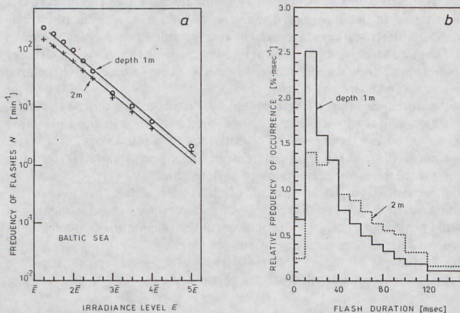
Fig. 1. Typical experimental data on near-surface flashing light in the open Baltic waters under conditions which favour strong focusing effect.
