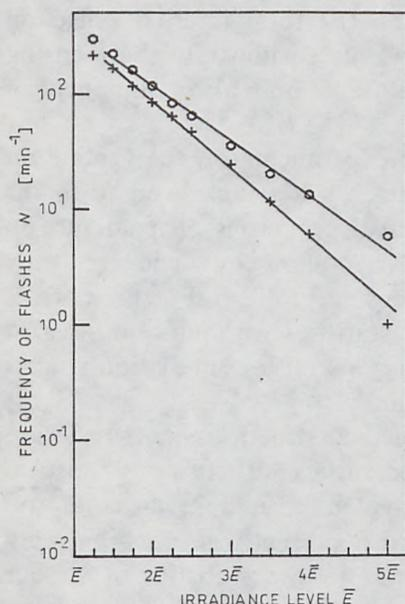
Fig. 7. Typical frequency distributions of flash intensity on a depth of 0.5 m measured in a water tank with generated surface waves exposed to the sunlight.
