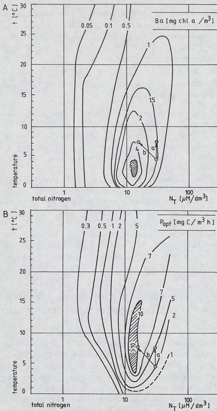
Figure 5: Approximate location of isolines: A - chlorophyll *a* concentration  $Ba = const$ ; B - optimum primary production  $P_{opt} = const$ , on diagrams  $t$  (temperature) versus  $N_T$  (total nitrogen concentration)
