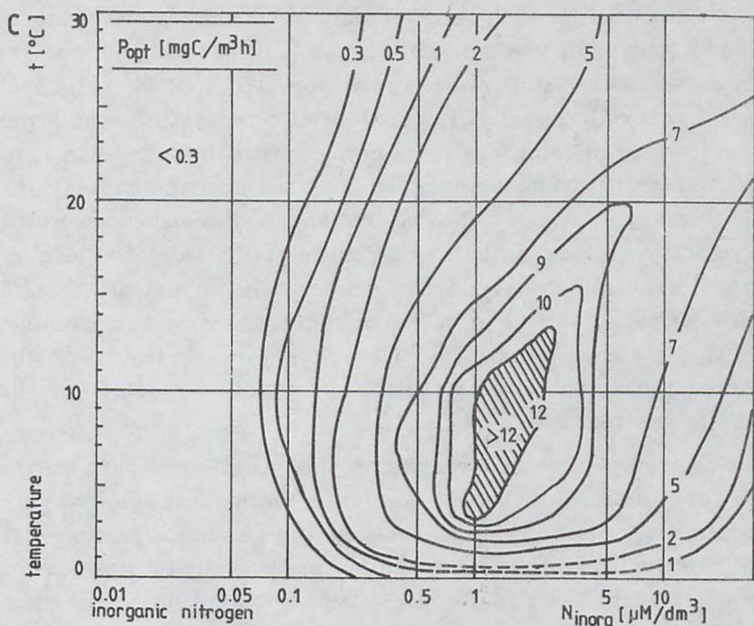
Figure 4: Approximate location of isolines: A - maximum assimilation number  $AN_{max} = const$ ; B - chlorophyll *a* concentration  $Ba = const$ ; C - optimum primary production  $P_{opt} = const$  on diagrams  $t$  (temperature) versus  $N_{inorg}$  (inorganic nitrogen concentration)
