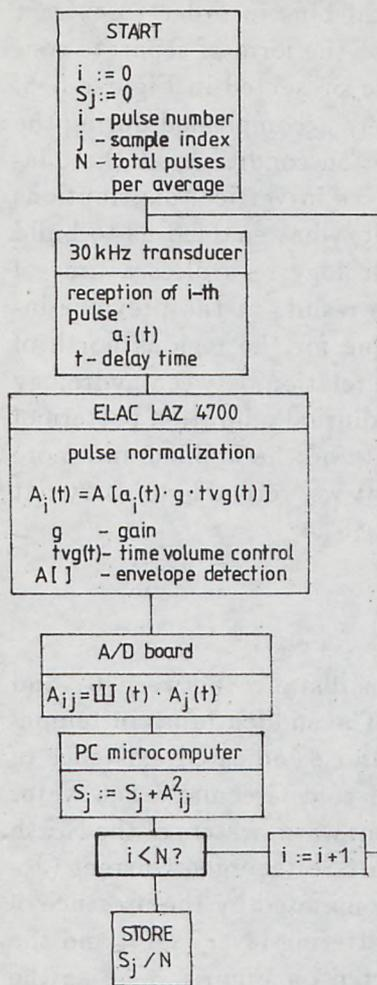
Figure 2: Diagram of the system for acoustic signal processing and recording used during the AREX-89 cruise
