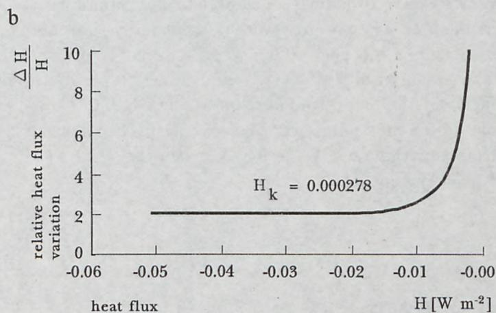
Fig. 1. Droplets mediated relative heat flux variation  $\Delta H/H$  versus heat flux  $H$  at the upper boundary of the modelled zone.  $H_k$  - heat flux between air and droplets. Unstable stratification (a), stable stratification (b)
