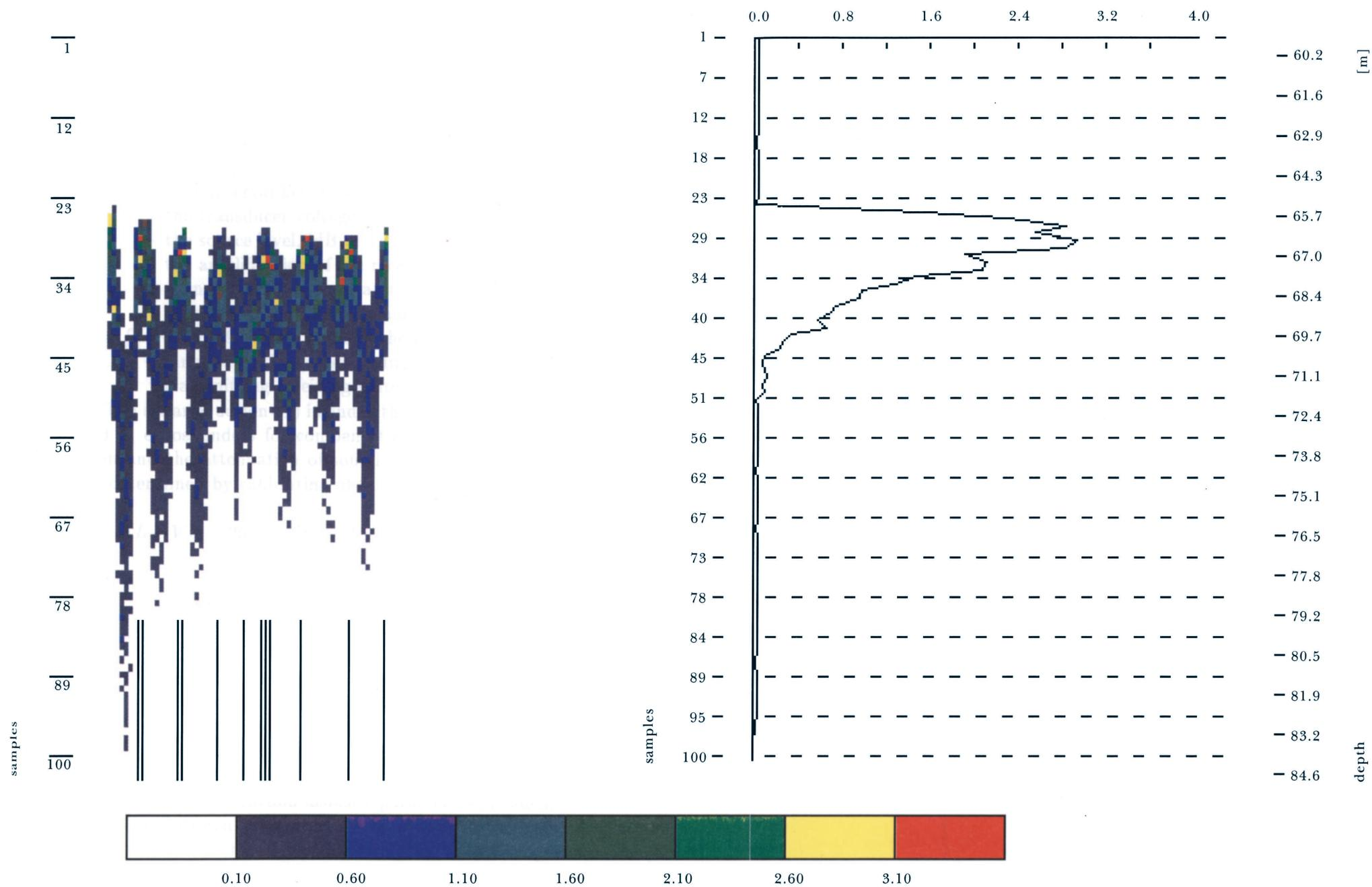
Fig. 3. Sequence of echoes and averaged profile as an example of the signal processing method
