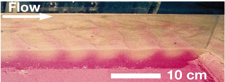
Fig. 1 Advective pore water transport in permeable sediment. Permeable sands exchange fluid and particles with the overlying water through advective pore water flows. In a laboratory experiment, red tracer dye shows the flushing of pore water from the sediment due to the advective pore water flows caused by unidirectional bottom flow (Photo by: M. Huettel).
